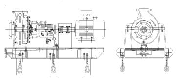
The pump type RAS (OH2) is a series of horizontal overhung centerline mounted, single stage, single suction heavy duty centrifugal pumps with volute design casings. The design of RAS complies with the American Petroleum Institute Standard Centrifugal Pumps For General Refinery Services, also known as API 610/ ISO 13709.
