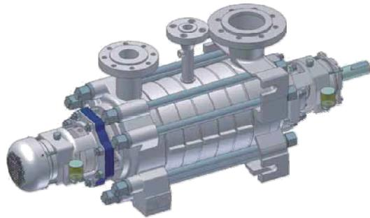
The RMDD is family of high pressure pumps is designed as per BB4 type. These pumps are also called ring-section pumps, segmental-ring pumps or tie-rod pumps, making it ideal for wide applications in high pressure boiler feed water, high pressure mine drainage, high pressure in water treatment plant.
